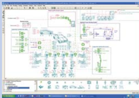
LMS Imagine.Lab Vehicle Dynamics can make a coupling between the vehicle model and the detailed model of key subsystems such as the steering system.
