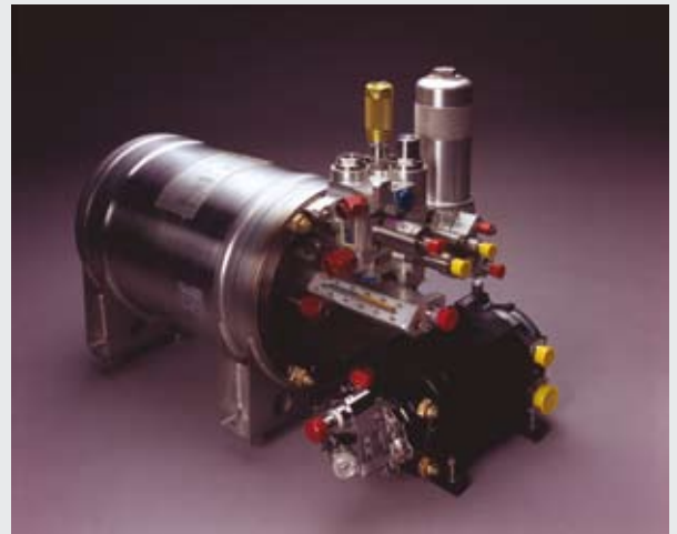
Local Electro Hydraulic Generation System (LEHGS) with its Electronic Control Unit (ECU)
